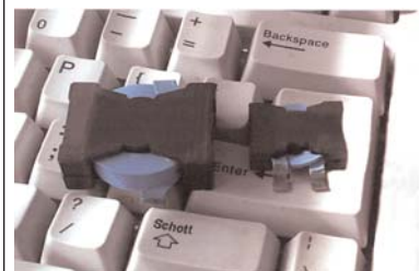
FIGURE 1 Planar Magnetics Assemblies Upper Photo => SMT units courtesy of Pulse Engineering Inc. Lower Photo => HWT™ Inductors courtesy of the Schott Corporation
